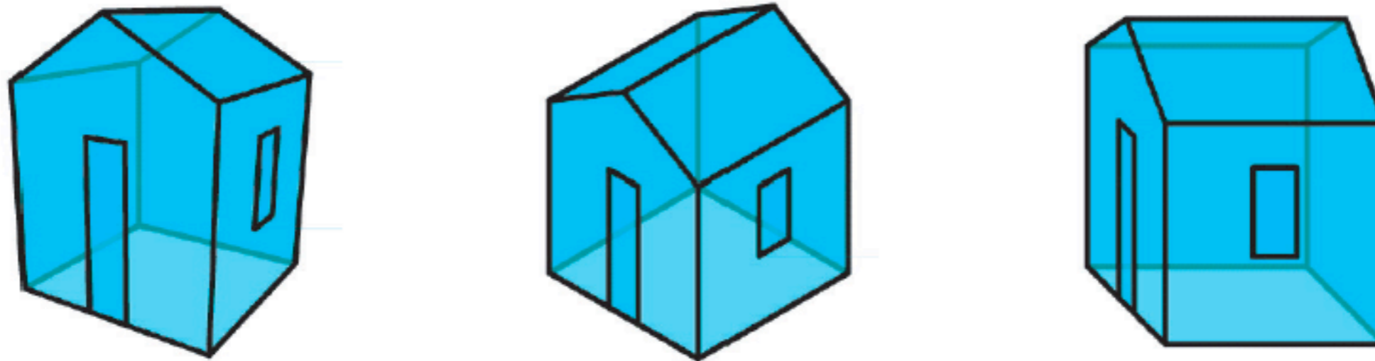
Figure 10.55 Projections exported as Flash files: (a) perspective oblique (b) parallel isometric (c) parallel cabinet
