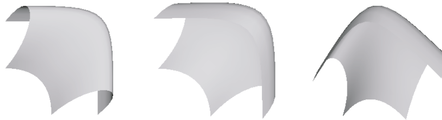
Figure 3: Some pictures of a new surface interpolating the same Hermite curves with constant oblique tangent vectors.
